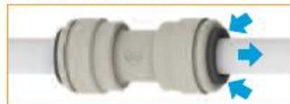
To disconnect, ensure the system is depressurized, push the collet square against the fitting. With the collet held in this position the tube can be removed.
