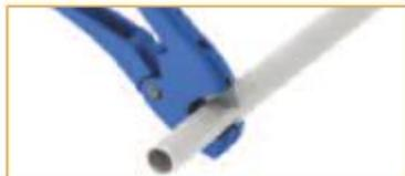
Cut the tube square and remove burrs and sharp edges. Ensure the outside diameter is free of score marks. For soft or thin walled tube we recommend the use of a tube insert.
